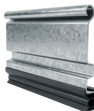
| GALVANISED STEEL BOTTOM BAR 142 x 28 mm · 2 mm thickness The lower part of the bottom bar includes a sealing rubber that improves performance. This bottom bar is compatible with the slats indicated above.
